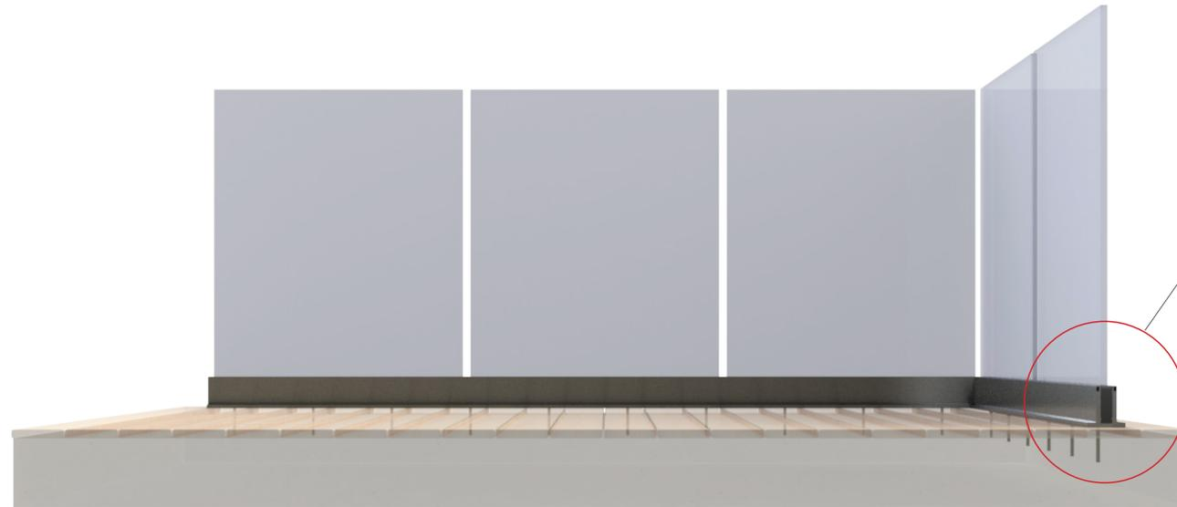
Elevation view fixed above finished floor level
