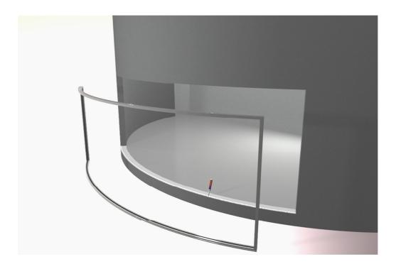
6. Place the frame in the correct position on the opening (remember to bring frame in from outside inward as the outside is longer than the inside).
