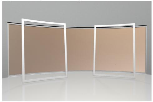
The way to insert doors onto the track is by lifting the door frame as high as possible into the top track, this allows the door to be able to line up above the bottom track and then be lowered onto it. As the top rail is not fixed yet, as you place the doors on the tracks make sure the top rail does not go too high and free from the doors.
