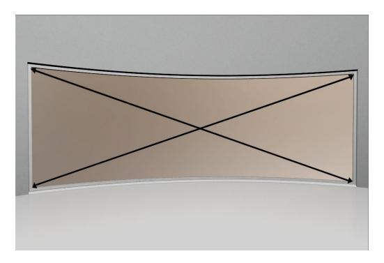
10.Fix the frame level to the opening on the SIDES only at this stage, leaving the top loose. NEVER drill the bottom rail! **NEVER drill or screw through the bottom rail**
