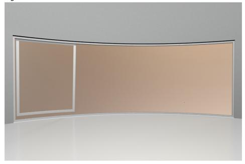
12.Fix the fixed doors in place by drilling in through the fixing spacers to the track. If there are no fixing spacers on the heights, fix these in place first on the height and then fix into the track.
