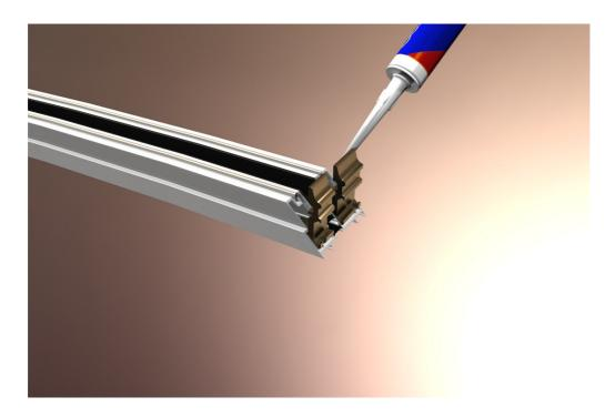
2. Connect top and bottom frame with uprights using the corner angles and allen inserts
