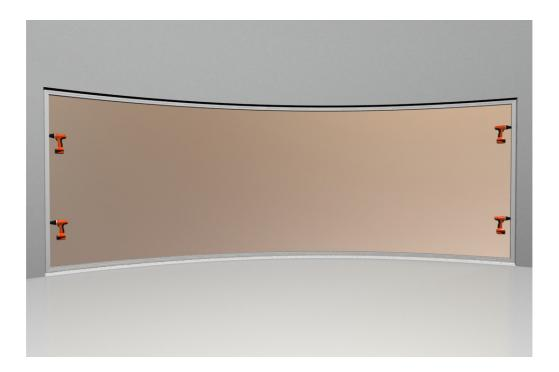
11.Get ready to insert the doors onto the track. Identify the fixed doors and insert them first. When inserting fixed doors make sure they have at least two fixing spacers already fixed to the bottom side. This will line them up height wise to align with the sliding doors.
