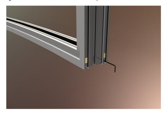
4. You may need to support the top frame with temporary supports so it does not sag until final fix.
