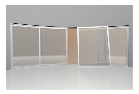
22. Fix the top track in place, in such a manner that it is correctly suspended at an equal height all along the opening and without putting its own weight onto the doors and so it does not apply any load or weight on the sliding doors underneath
