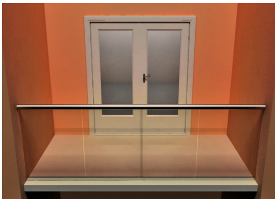
Balcony 1 Balustrade fixed between two walls
