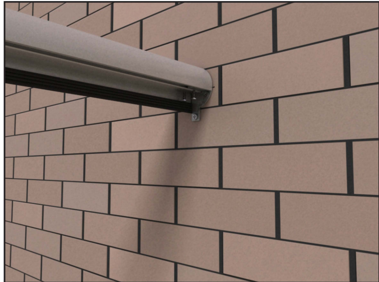
22 Drill 4mm holes through brackets in the handrail. Fix the handrail to the wall bracket using the No. 10 x 3/4" S/tapping screws
