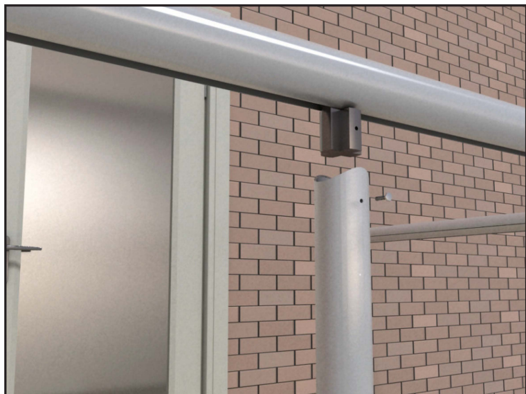
24 Fix the post into the post connector using the M5 screw provided
