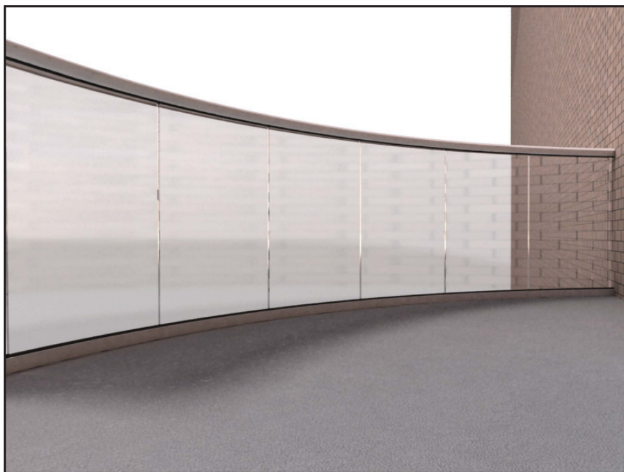
75 * Once the silicone is dry on the bottom rail remove the temporary beads and replace the full length curved bead.
