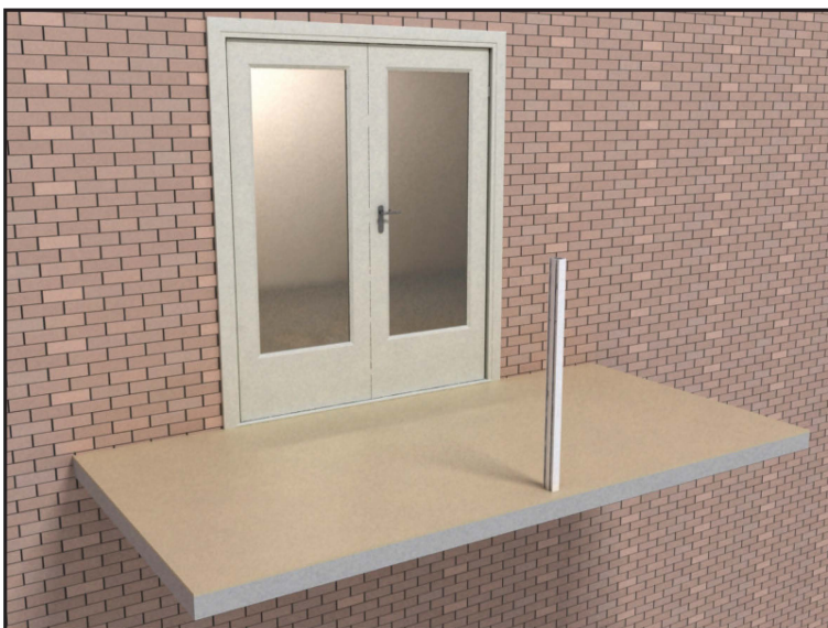
17 Check that the system cover post is sitting on finished floor level.
