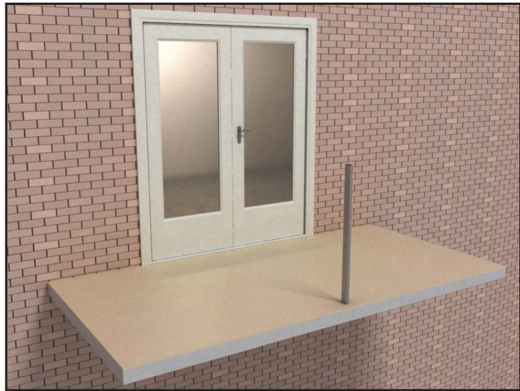
14 Finish the flooring, decking, screed, floor finish etc. to the required height. This should conceal the base plate and bolts
