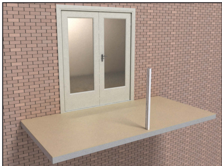
18 Aluminium post in position
