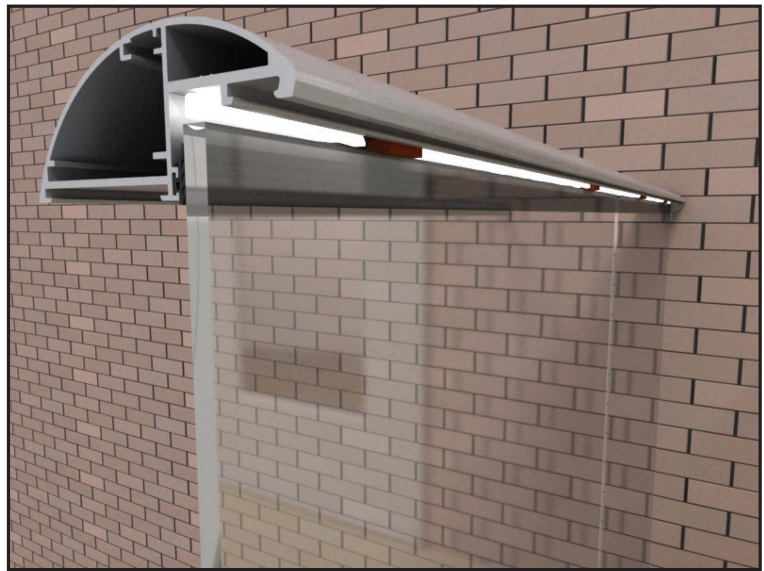
52 Remove the temporary glazing beads and rubber gaskets
