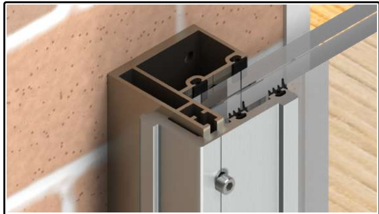
18) The glass is now fully supported.
