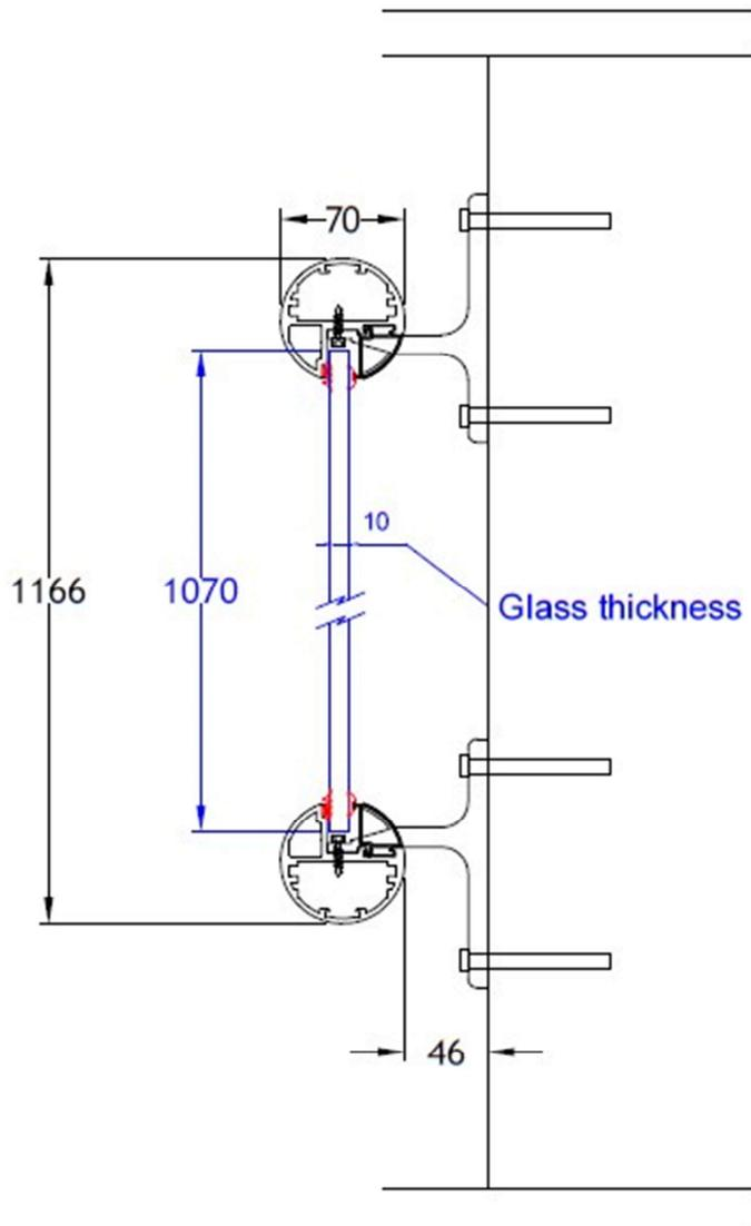
Typical section & handrail profile moment of inertia
